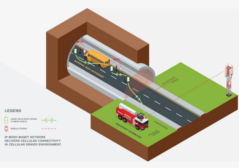
Mesh radio connected to cellular modem on the exterior - in this example the command vehicle outside the entrance of the tunnel. The exterior radio connects to the other radios in the tunnel (cellular denied), thus giving cellular access to devices connected to each radio.
